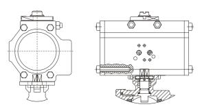
ISO direct mount for actuator assembling directly.
