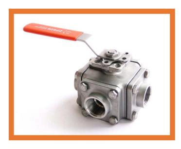
ZIPSON'S 501T, multi-way ball valve with ISO direct mount is a smart way to save the cost on pipe line and space. With T/L/X/I-port for 3/4/5way block body type, and will be easy to find a suitable type for any application. The 501T designed with ISO direct mount for assembling the actuator directly.
