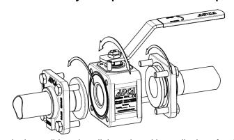
Loose body flanges make it possible to install the valve without aligning of welded end connections. After installation the valve can rotate on 360° for the desired orientation.
