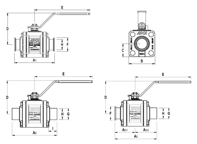
Tube weld easy and quick installation - optional
