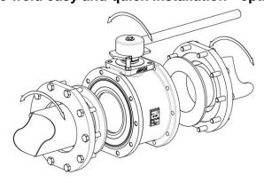
Loose body flanges make it possible to install the valve without aligning of welded end connections. After installation the valve can rotate on 360° for the desired orientation.
