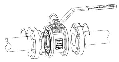
Loose body flanges make it possible to install the valve without aligning of welded end connections. After installation the valve can rotate on  $360^{\circ}$  for the desired orientation.
