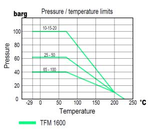
Working pressure may be limited by the valve connections.
